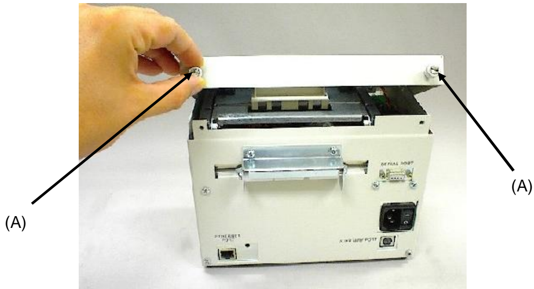
Figure 16 Removal of top cover
